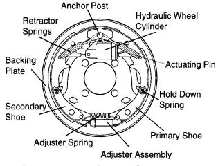
Figure 57. Hydraulic Brake Components
